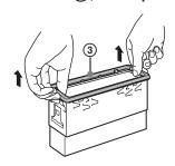
2 Insert both release keys ② until they click, and pull down the bracket ①, then pull up the unit to separate.
